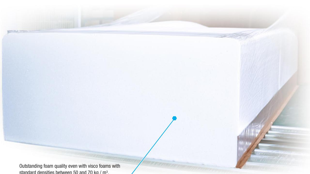
Outstanding foam quality even with visco foams with standard densities between 50 and 70 kg / m<sup>3</sup>.
