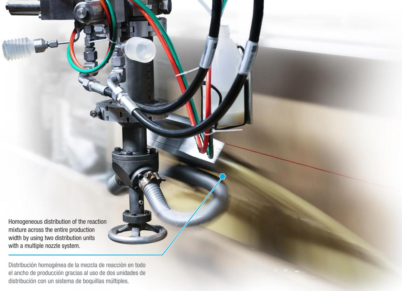
Homogeneous distribution of the reaction mixture across the entire production width by using two distribution units with a multiple nozzle system.
