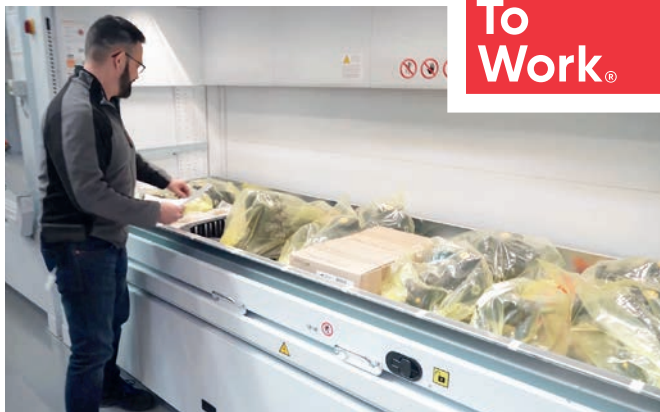
The automated storage towers make work in the warehouse not only more efficient, but also more ergonomic.
