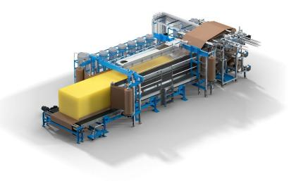
JFLEX evo: The ultra-compact system with a 54 m<sup>2</sup> footprint and a height of three meters saves valuable production space.
